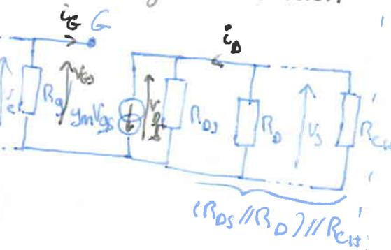
(2)  $V_{G_{S_0}} = -R_S I_{D_0} \Rightarrow$  (3)  $I_{D_0} = I_{DSS} \left(1 + \frac{R_S I_{D_0}}{|V_P|}\right)^2$
