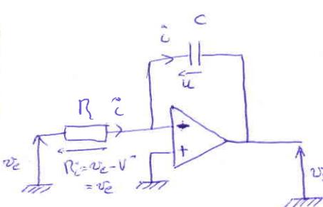
$$V^- = \frac{\frac{V_E}{j \omega C} + \frac{V_s}{R}}{\frac{1}{j \omega C} + \frac{1}{R}} = 0 \Leftrightarrow \frac{V_E}{j \omega C} + \frac{V_s}{R} = 0.$$
